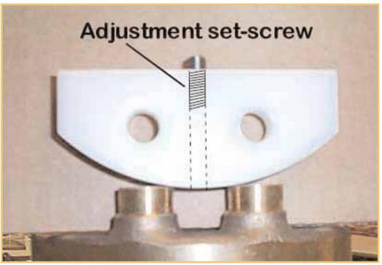
Please confirm that the narrowest gap between the tank guides and the retraction tube wall is **0.5mm**. Adjust if necessary.
